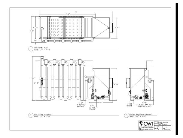
Figure 9. The Dimensions of the GEM System installed at the rendering plant
