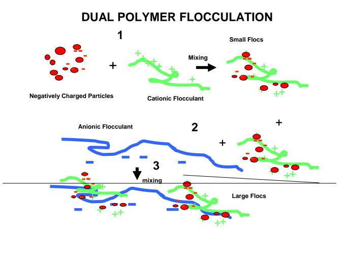
Figure 5. Dual polymeric flocculant approach.
