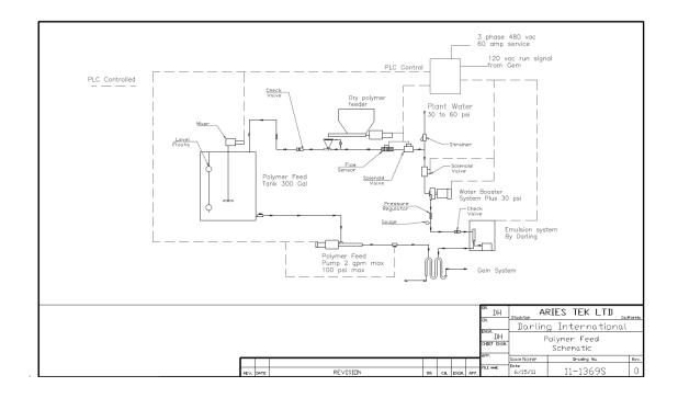
Figure 8. Automatic feed System for the granular flocculants
