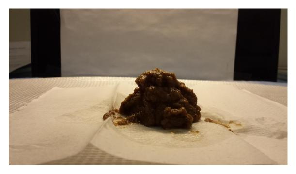
Figure 1 – Sludge Skimmed from GEM System at Rendering Facility
